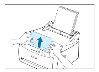
If paper is jammed in the face-up output slot, carefully remove the paper as shown.
